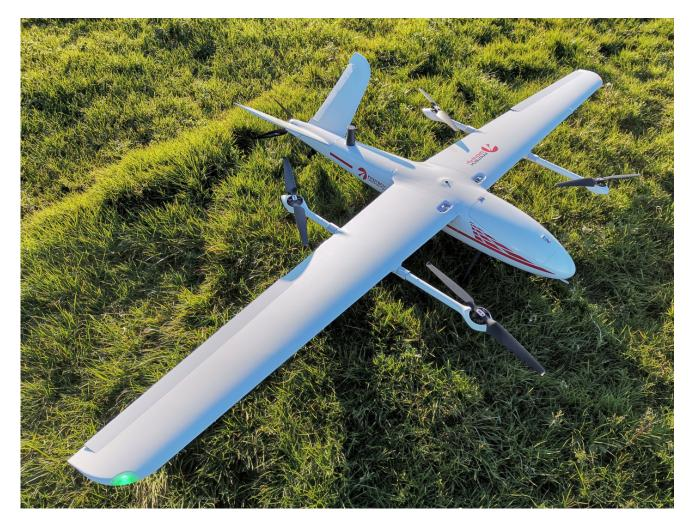
Survey and Mapping - RGB Camera Precision Agriculture - Multispectral Camera Surveillance - Thermal Camera
